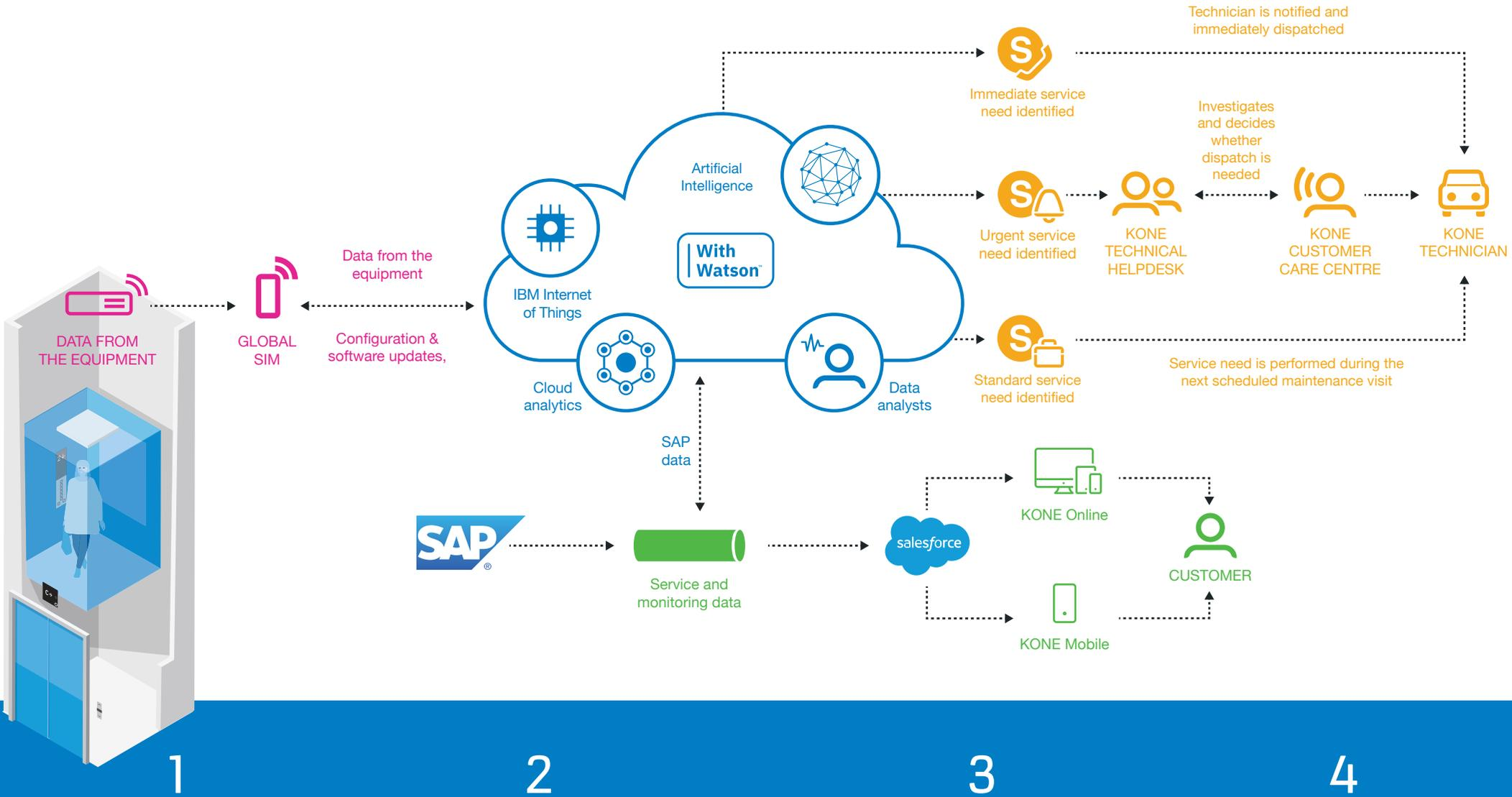
Information on the key operating parameters, usage statistics and faults is sent in real time to KONE's cloud service, where the analytics are located.
