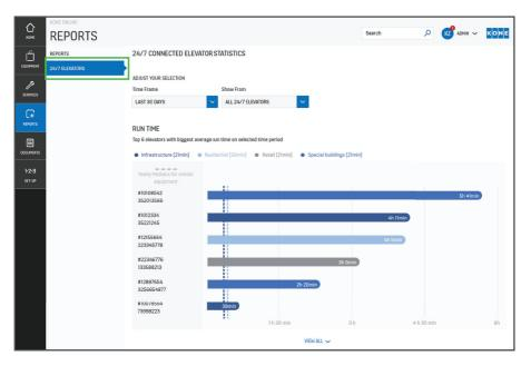
Elevators connected with KONE 24/7 Connected Services will show how long the equipment has been in operation and how many starts have occurred during the selected time period.
