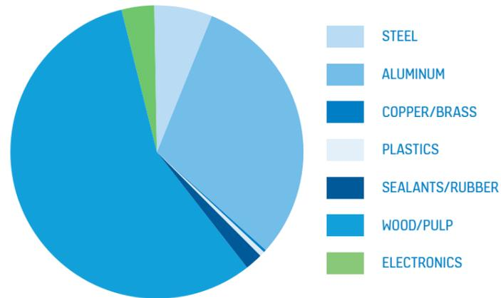
Figure 8. Material structure example for KONE Hermetic Door 30
