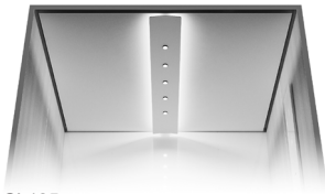
CL195 Direct lighting: LED spot Indirect lighting: LED strip Finishing: PP10FT
